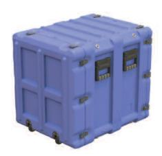
Amazon design skills have also been applied to produce a new generation of 19 inch racks to protect electronic, IT and telecommunications equipment against climatic extremes and rough handling in field conditions. Amazon Racks combine the tough resilience of a rotomoulded case with a lightweight stainless steel rack frame and a unique elastomeric suspension system.
