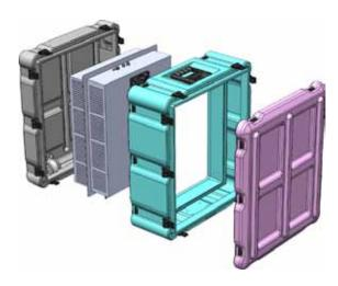
The Cooler Collar for Amazon 19-inch racks utilises the patented Amazon lip and tubular silicone gasket to create an airtight and waterproof seal to allow the AC unit to function in extreme conditions. Where a greater cooling requirement is needed, two Cooler Collars with AC units can be fitted to both the front and rear of the rack.
