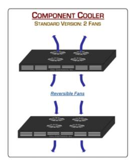
**2-Fan Unit (2FN):** This unit ships with two fans mounted so the air flows from the bottom of the unit through to the top. The fans are easily reversible by pulling them from their mountings, flipping them, and refastening them by pulling the mounts through the mounting holes on the fans. You can also change the orientation of the fans to use any of the four fan openings.
