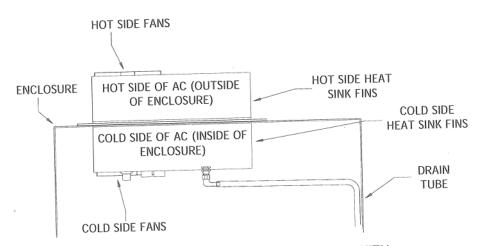
HORIZONTAL INSTALLATION OF 800 BTU UNIT WITH INTERNALLY MOUNTED DP-141H DRIP PAN AND DRAIN TUBE
