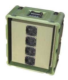
The maximum depth of equipment that can be fitted in a 610 mm rack (when not in the lowest position) is 750 mm. The COOL-COLLAR can also be attached to a rack without an AC unit installed, to extend the maximum depth that can be used to 800 mm.
