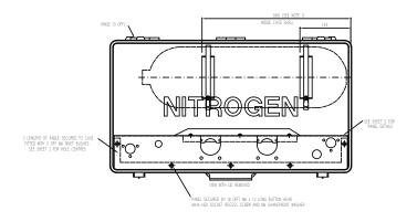
The case interior needed carefully constructed supports, partitions and fixings. The internal also had to be multi layered due to the height variation of the valves.
